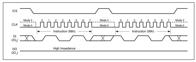
Figure 5b. Enable Reset and Reset Instruction Sequence
