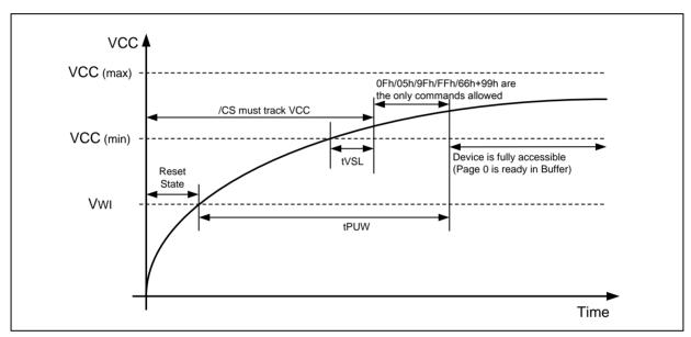
Figure 30a. Power-up Timing and Voltage Levels
