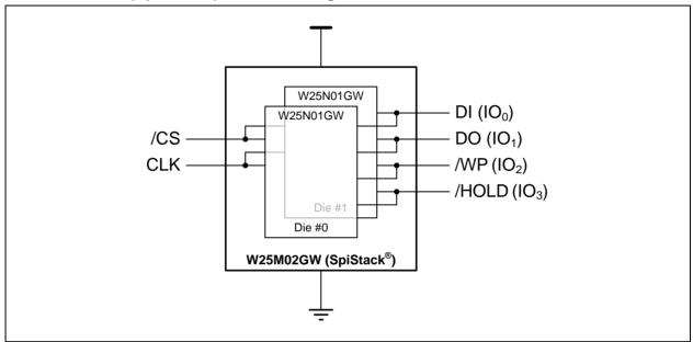
Figure 2a. W25M02GW Device Configuration
