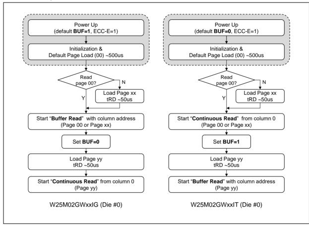
Figure 2c. W25M02GW Flash Memory Operation Diagram
