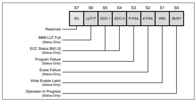
Figure 3c. Status Register-3 (Address Cxh)
