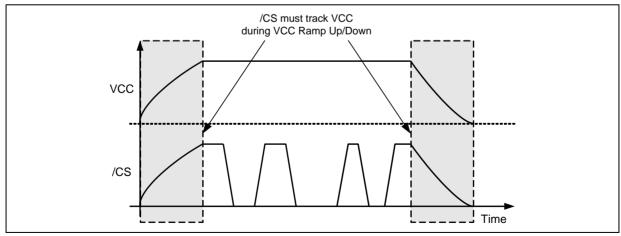
Figure 30b. Power-up, Power-Down Requirement
