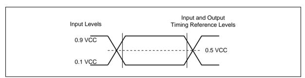
Figure 31. AC Measurement I/O Waveform
